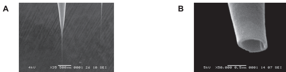
Figure 3.2. Scanning electron imaging of borosilicate glass pipettes produced with a pipette puller (A). (B) Higher magnification image of tip in (A). Scale bars are 500 \mu\text{m} and 500 nm, respectively.
